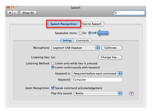
3. Use the Microphone menu to select your microphone. Clicking on Calibrate will open a window where you can use the slider to adjust the microphone input level.
